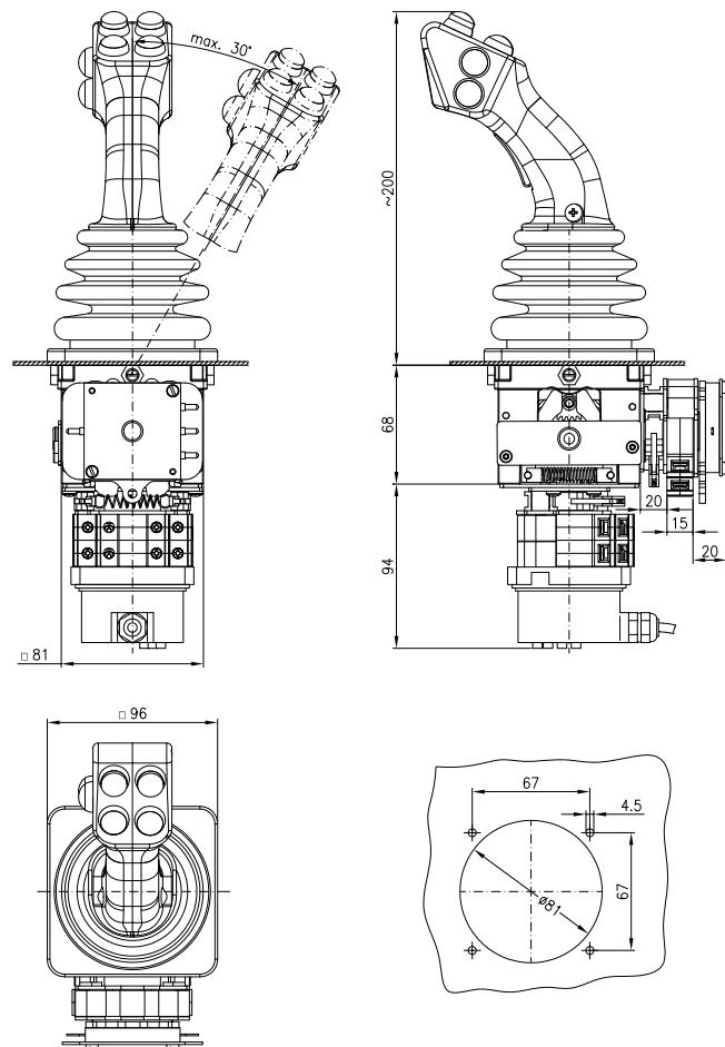
The hollow special-alloy lever (VNSO 8 mm, NNSO 12 mm diameter) allows to assemble a variety of grips and the wires can be routed through the joystick. Grip rotation may come in different grip versions. Due to the special coupling design it is easy to flange different potentiometers as well as optoelectro-
