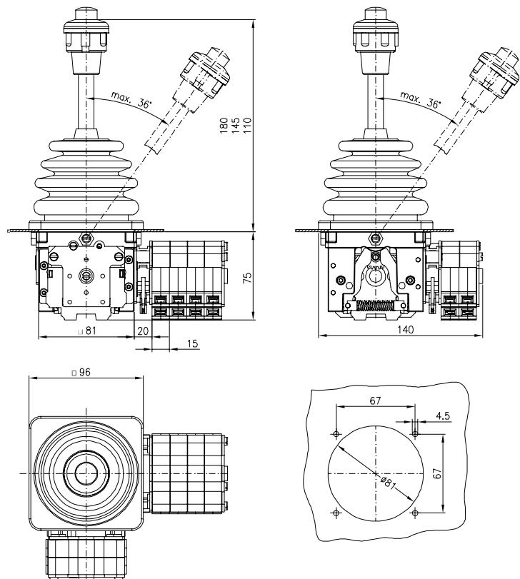
Our allrounder VNS0 and our special type NNSO. Both the VNS0 and the NNSO are very robust joysticks with aluminium pressure casting consoles and metal gears. Their resistance against ozone, UV radiation, oil and maritime climate makes them especially suitable for heavy operations and in Ex-areas. They are available both as single and compound axis drives. The intelligent modular design allows customized
