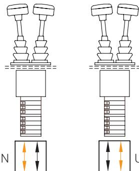
Potentiometer and encoder coupling
