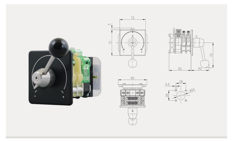
The NS00 and NS20 are very robust rotary switches with 6 and 12 mm diameter metal square shaft, aluminum nameplate, and cam-actuated contacts. The switch contacts, embedded in double contact modular blocks, with positive break by cam discs, are available in a gold-plated version for low voltage, as a silver contact for standard applications,
