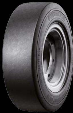
With its slick tread and the closed shoulders, the SH12 is an excellent solution when low energy consumption, high driving comfort through smooth running and protection against damages are required.
