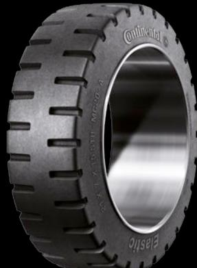
If low passage heights, heavy loads and maintaining high levels of traction are required, the Continental MC20 proves its strengths. Despite its compact design, the MC20 has a profile with a smooth tread. Therefore heavy loads can be transported safely on almost all surfaces.
