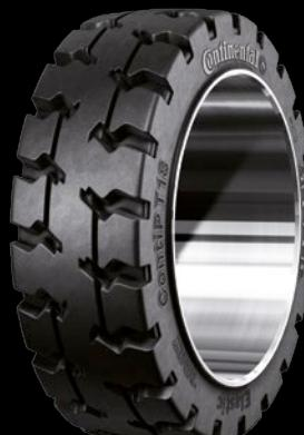
The ContiPT18 transports the superior driving forces of a super elastic tire onto a Press on Bands. With its special tread it achieves excellent levels of traction, combined with high loads.
